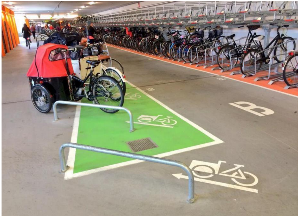
Example of a 'half-height' stand in Malmo, Sweden, which is intended to accommodate non-standard bicycles. It provides the space needed for longer bicycles and pavement markings help reduce tripping hazards. Photo credit: Kevin Hickman
