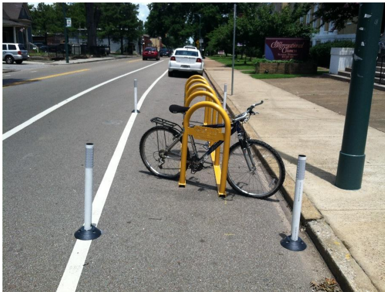
Example of a bicycle corral in Memphis, Tennessee. Image credit: City of Memphis
